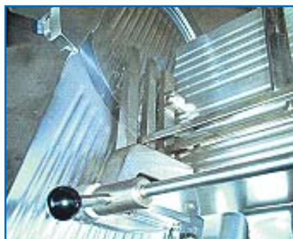
A stainless-made products pusher is clean and it can hold the products more than before.
